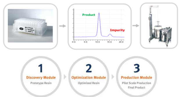
Figure 6. The 3 stages of a typical custom design modular study. It covers the stages of Screening (1), Optimization (2) and Scale-up (3).
